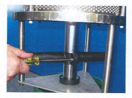
Figure 25: Removal of the water motor
