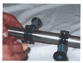
Figure 32: Nozzle removal
