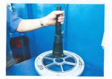
Figure 23a: Remove reverser housing
