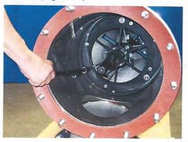
Figure 15: Loosening clamp nuts
