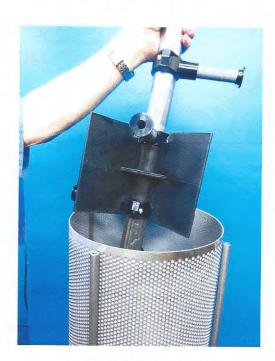
Figure 26: Rotor removal
