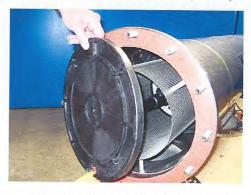
Figure 12: Removal of prestrainer cap.
