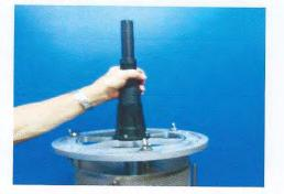
Figure 22: Upper bulkhead removal
