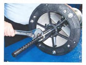
Figure 28: Removal of the retaining nut
