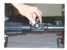
Figure 19: Removing pawl retainer cap
