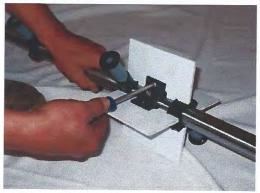
Figure 30: Removing the rotor paddles
