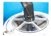
Figure 23: Remove reverser housing screws
