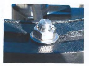
Figure 16: Clamp bolt in unlocked position
