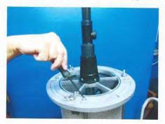
Figure 21: Removal of allen screw
