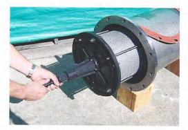
Figure 17: Internal Assembly Removal
