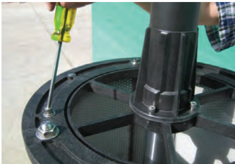
Figure 21: Removal of allen screw
