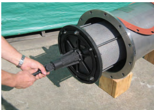
Figure 17: Internal Assembly Removal
