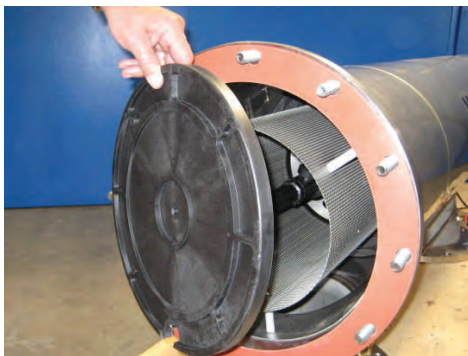
Figure 12: Removal of prestrainer cap.
