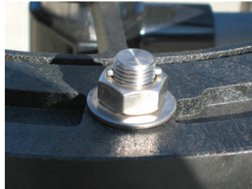
Figure 16: Clamp bolt in unlocked position
