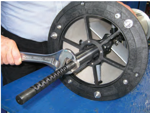
Figure 28: Removal of the retaining nut
