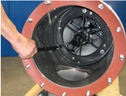
Figure 15: Loosening clamp nuts
