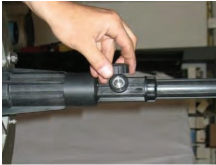
Figure 19: Removing pawl retainer cap
