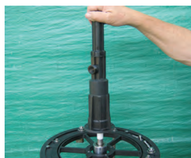
Figure 23a: Remove reverser housing
