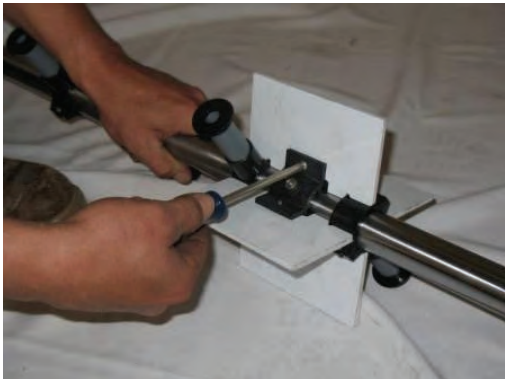
Figure 30: Removing the rotor paddles
