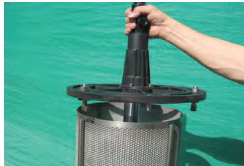
Figure 22: Upper bulkhead removal
