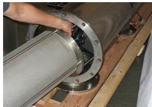
Figure 18: Supporting the internal assembly
