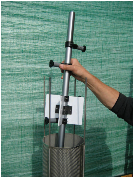
Figure 30 Lifting collector tube
