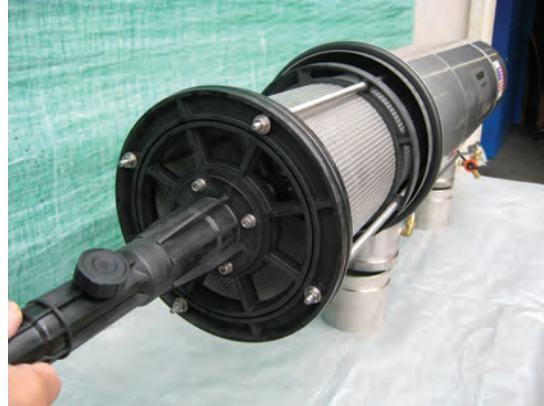
Figure 14 Pulling Internal Assembly
